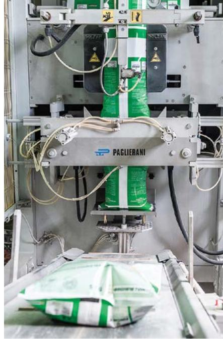
**FINOMIX** dry mortars are produced at the company's facilities in Chordaki, Chania, in a modern, fully automated production plant with a capacity of 500 tons per day. The plant is designed in a vertical arrangement in order to increase productivity and reduce energy consumption.
